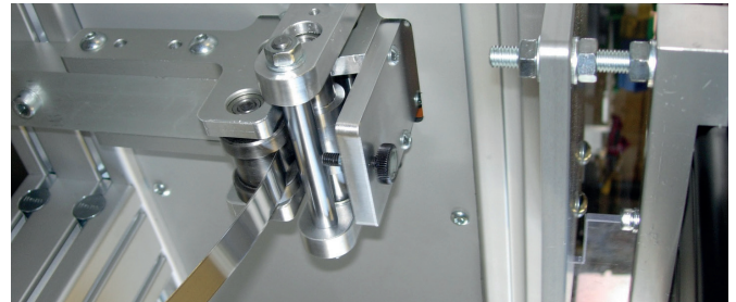
SS strip, linear fed laser marking - aerospace
